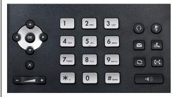
The four-way keypad at the top left is used to navigate the phone's menu system, and the four keys also double as shortcuts. Pressing UP displays the call history, and pressing DOWN displays the number directory, LEFT and RIGHT select the line appearance key to use for making an outgoing call.
