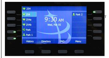
There are five keys on each side of the screen, and four keys below the screen. The keys along the side of the screen are programmable, and change depending on the configuration of your phone. In this example, there are three line keys and three park buttons. The bottom four keys on the right side have not been programmed, so they are blank.
